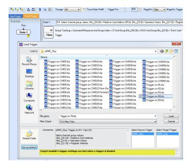
Each trigger contains a list of the fields within the command or response packet type you selected. Numeric fields, such as a device's Relative Card Address (RCA), allow direct input in the radix of your choice. Fields with a predefined list of options provide a pop-up selection list. The trigger groups corresponding to each packet field are identified in the comment header.
